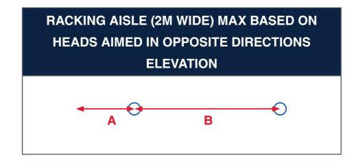
Luminaire spacing for racking aisle
